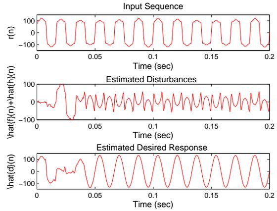
Fig. 20. The input signal to the filter and the estimated signal at the output of the filter, filter order=100.
