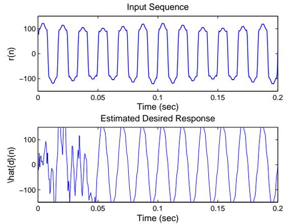
Fig. 16. The input signal to the filter and the estimated signal at the output of the filter, filter order=100.
