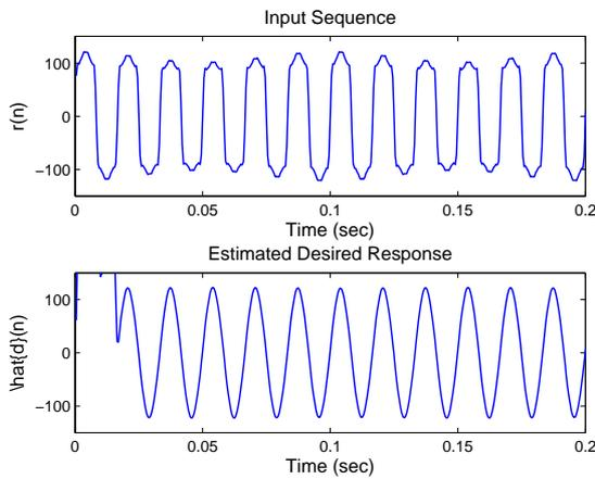
Fig. 15. The input signal to the filter and the estimated signal at the output of the filter, filter order=35.
