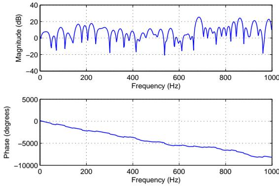
Fig. 14. The frequency and phase response of the filter design estimating the desired signal, filter order=100.
