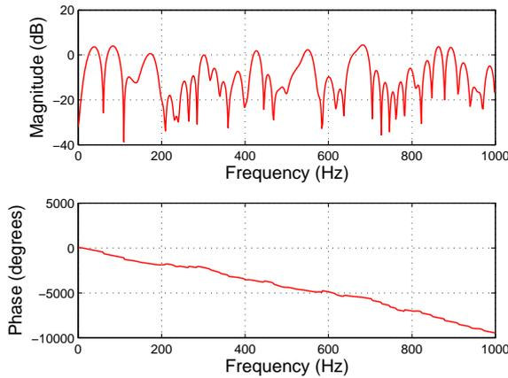
Fig. 18. The frequency and phase response of the filter design estimating the desired signal, filter order=100.
