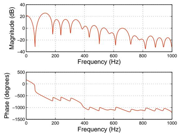
Fig. 17. The frequency and phase response of the filter design estimating the desired signal, filter order=35.
