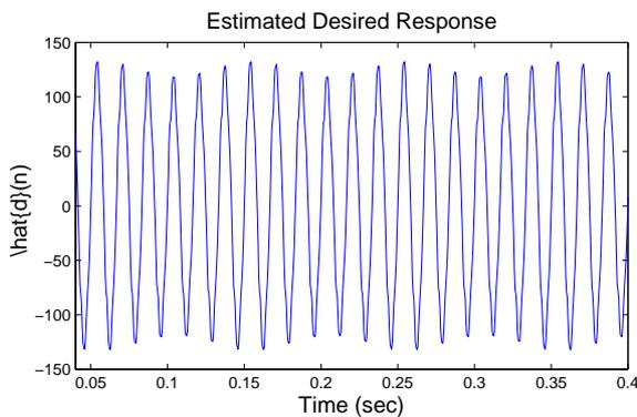
Fig. 11. The estimated signal desired signal in presence of large harmonics and flickers for the first algorithm.
