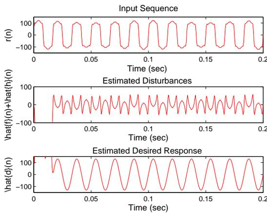
Fig. 19. The input signal to the filter and the estimated signal at the output of the filter, filter order=35.
