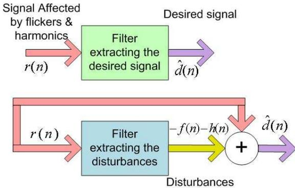
Fig. 1. The block diagram representing the two filter designs used to remove the disturbances from the received signal.
