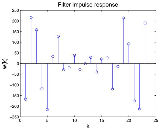
Fig. 4. The the impulse response for a filter of order 23 estimating the desired signal.
