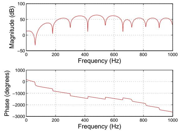
Fig. 9. Frequency and phase response of the filter outlined in Fig. 8.
