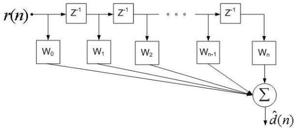
Fig. 2. The finite impulse response used to estimated  $\hat{d}(n)$ .
