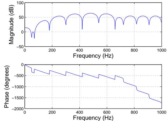
Fig. 5. Frequency and phase response of the filter outlined in Fig. 4.
