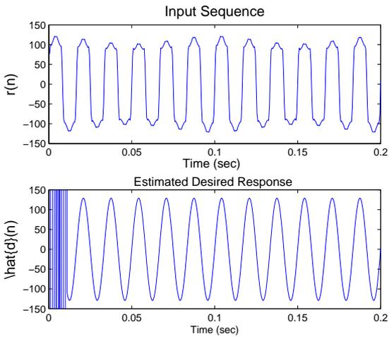
Fig. 7. The lag required for the filter response to stabilize.
