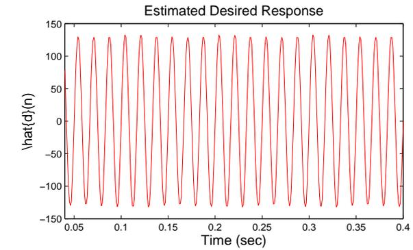
Fig. 12. The estimated signal desired signal in presence of large harmonics and flickers for the second algorithm.
