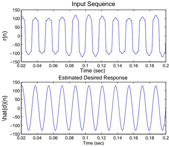
Fig. 6. The input signal to the filter and the estimated signal at the output of the filter represented in Fig. 4.
