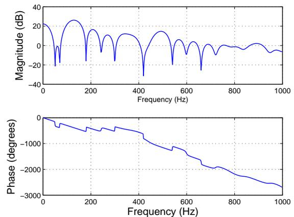
Fig. 13. The frequency and phase response of the filter design estimating the desired signal, filter order=35.
