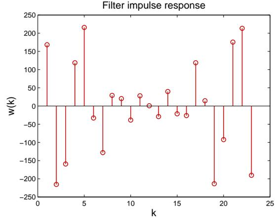
Fig. 8. The the impulse response for a filter of order 23 estimating the disturbances.
