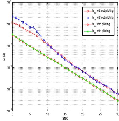
Fig. 2. Average MSE for  $h_{ba}$  and  $h_{aa}$  for shifted modulation
