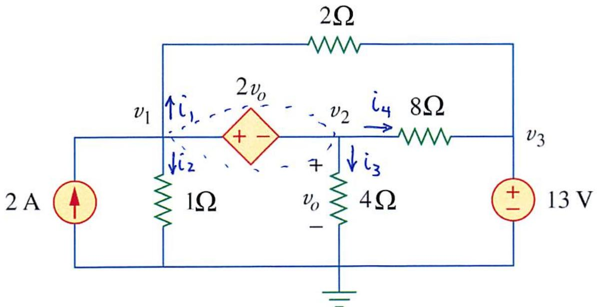
$$KCL @ SN \quad 2 = i_1 + i_2 + i_4 + i_3$$
