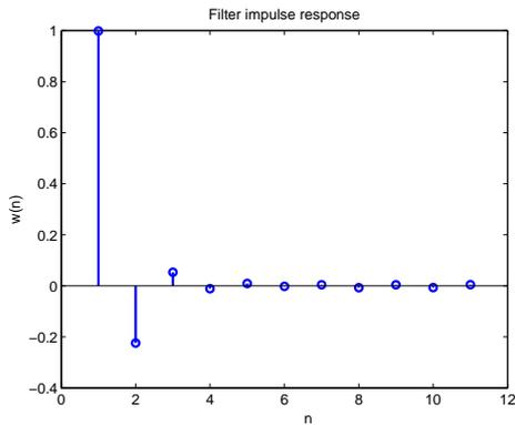
Fig. 4. The impulse response of the Wiener equalizer with  $\xi = 2.9$  and  $\sigma_n^2 = .001$ .
