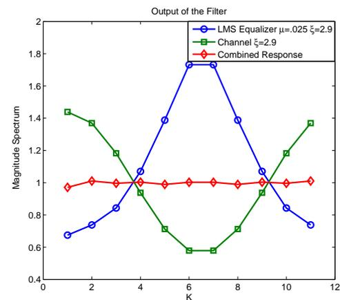
Fig. 11. The magnitude spectrum of the LMS equalizer, the channel, and the combined system.
