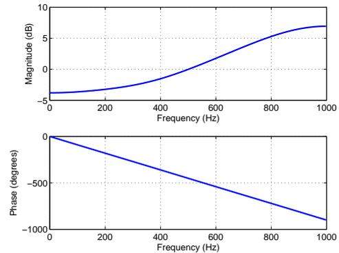
Fig. 10. The magnitude and phase response of the LMS equalizer.
