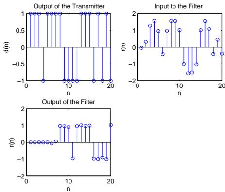
Fig. 8. The output of the transmitter, the input to the filter, and the output of the filter for the LMS equalizer.
