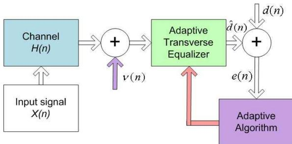
Fig. 1. The block diagram representing the two filter designs used to remove the disturbances from the received signal.
