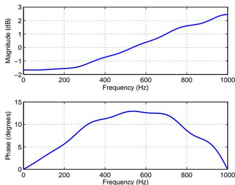
Fig. 5. The magnitude and phase response of the Wiener equalizer.
