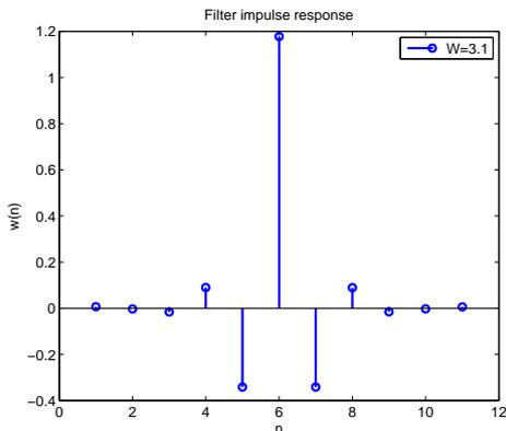
Fig. 9. The impulse response of the LMS equalizer with  $\xi = 2.9$  and  $\sigma_n^2 = .001$ .
