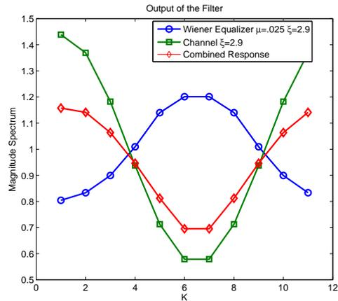
Fig. 6. The magnitude spectrum of the Wiener equalizer, the channel, and the combined system.
