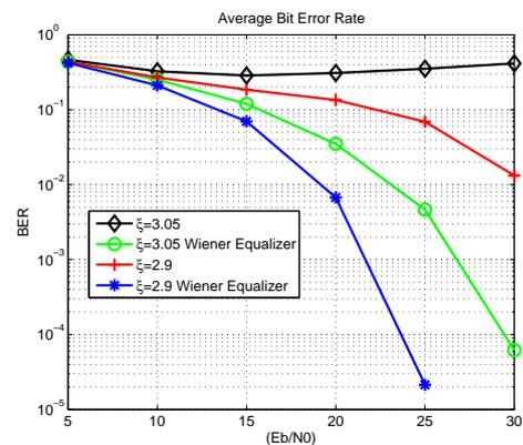
Fig. 7. ABER plots for digital system equipped with and without the Wiener equalizer at  $\xi = 2.9$  and  $\xi = 3.05$  distortion levels.
