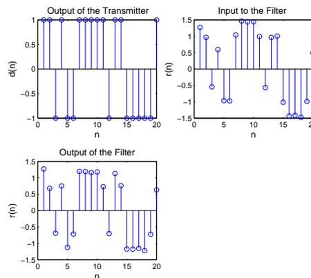
Fig. 3. The output of the transmitter, the input to the filter, and the output of the Wiener equalizer.
