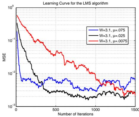
Fig. 12. MSE for the LMS equalizer at  $\mu = .075$ ,  $\mu = .025$ , and  $\mu = .0075$ .
