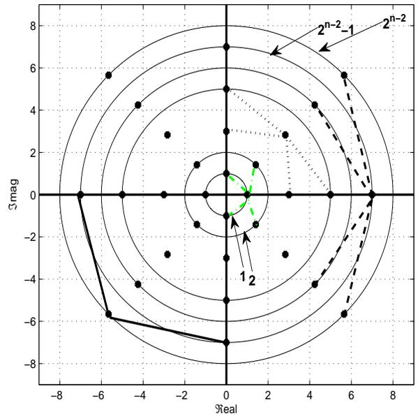
Fig. 1: Schematic illustration of the circular QAM constellation [20].
