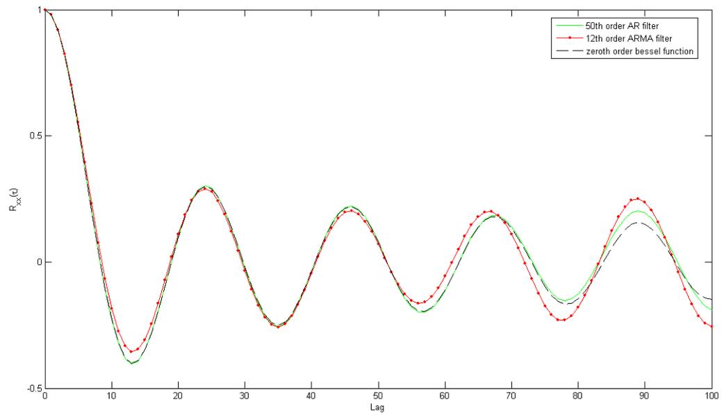
Fig. 3. Autocorrelation for ARMA(12) and AR(50) filters
