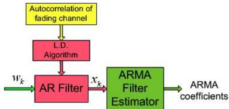
Fig. 1. Block diagram representing the information flow to determine the coefficients of the ARMA filter
