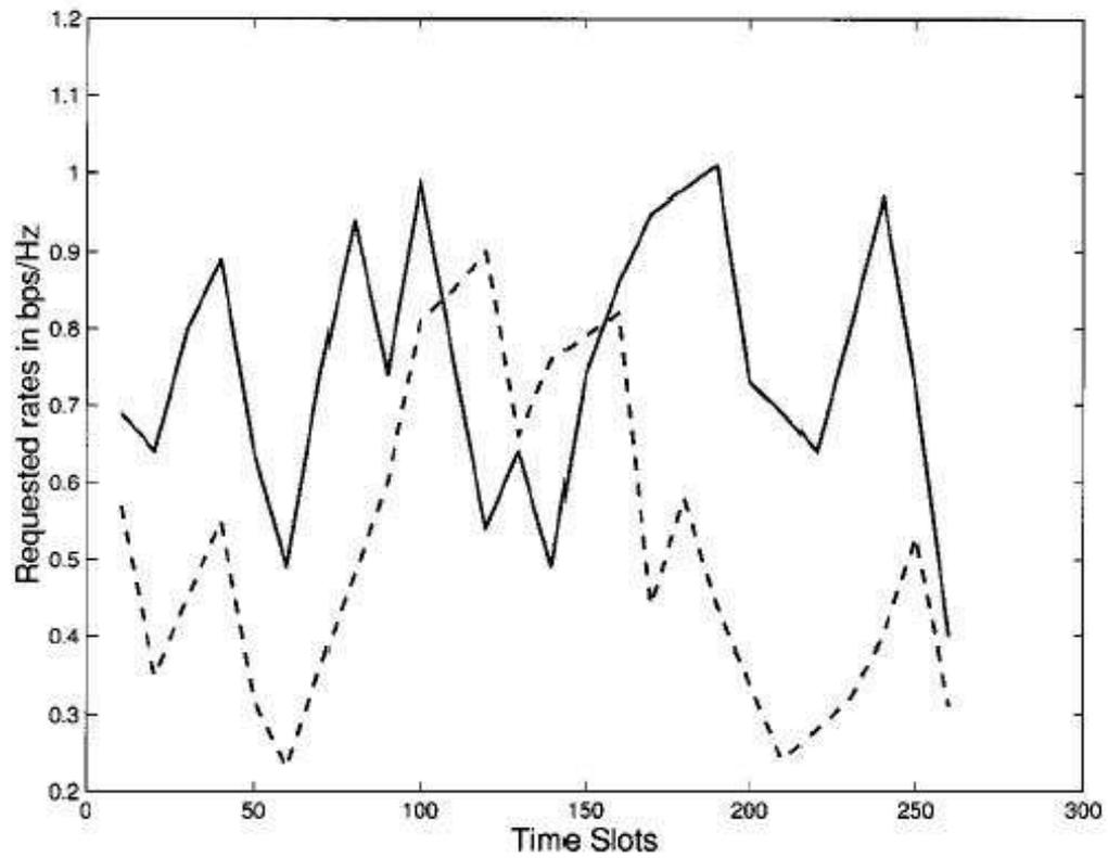
Fig. 3. In general, with asymmetric user channel statistics, the scheduling algorithm serves each user when it is near its peak within the latency time scale  $t_c$ . [1]
