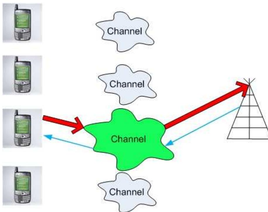
Fig. 1. Multi user diversity provides transmission to the user with the best channel at any given time.
