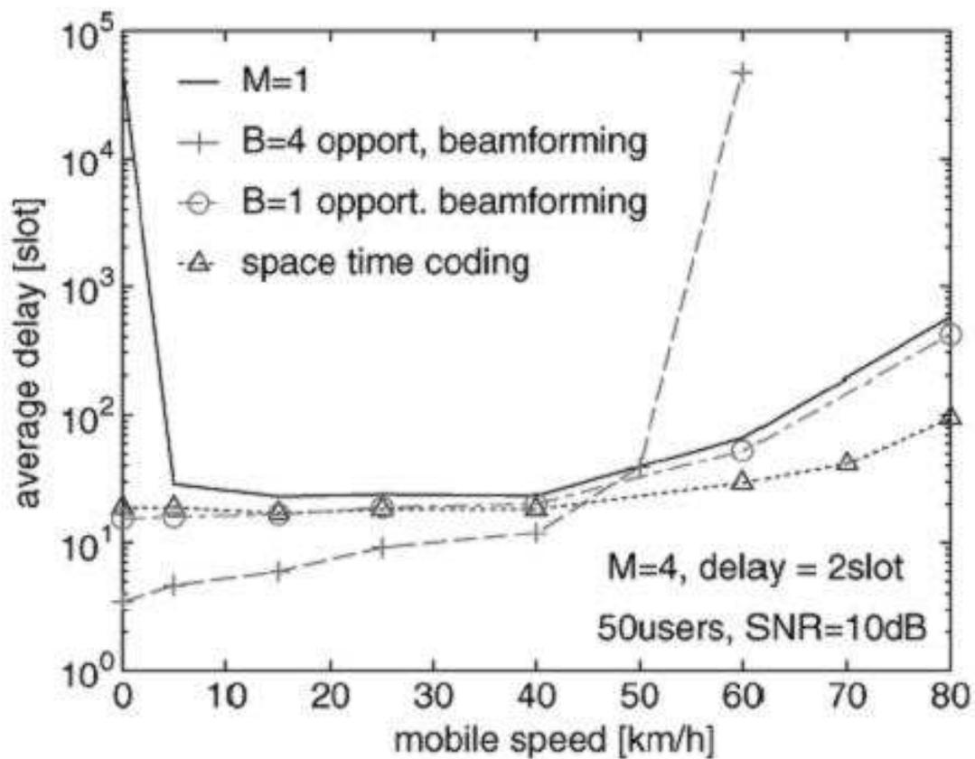
Fig. 7. Average delay versus mobile speed for the case of  $K = 50$  users and  $M = 4$  transmit antennas. The cases of random beamforming with  $B = 1$  and  $B = 4$  beams, and STC are compared. The case  $M = 1$  (single antenna) is also included for comparison. [3]
