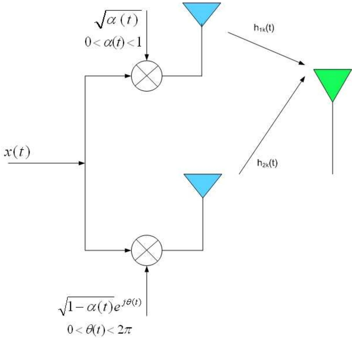
Fig. 5. The same signal is transmitted over the two antennas with time-varying phase and powers. [1]
